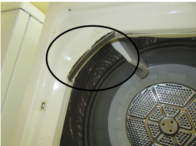
The dryers clothes drum appears to be out of alignment and has cut through the unit's casing on the interior of the door to the unit. Some resting and paint chipping is noted on the top of the dryer unit.
