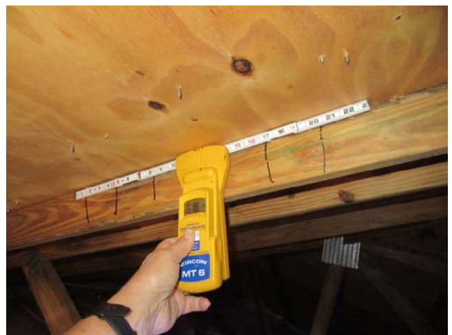
Roof nailing pattern of 8pn nails installed 6" oc center in the field and 6" oc center on the edge is determined with the use of a Zircon MT6 metal detector.
